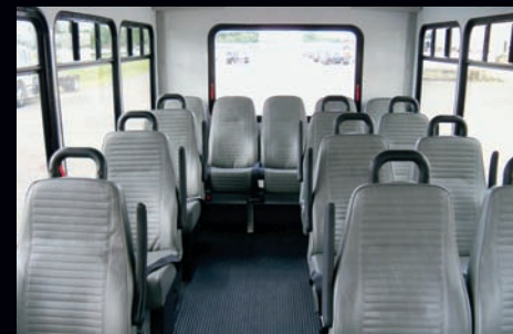
Optional 13 passenger capacity with mid back seats, top seat mounted grab handles and armrests. Also shown, complete FRP interior for long lasting durability.
