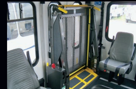
Optional ADA wheelchair lift mounted in the rear of the bus
