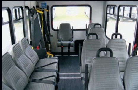
Optional wheelchair accessible floor plan with mid back seats, top mounted grab handles and armrests. Also shown, complete FRP interior for ease of cleaning.
